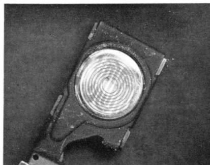
Two CDS elements of different sensitivity give more accurate response.
