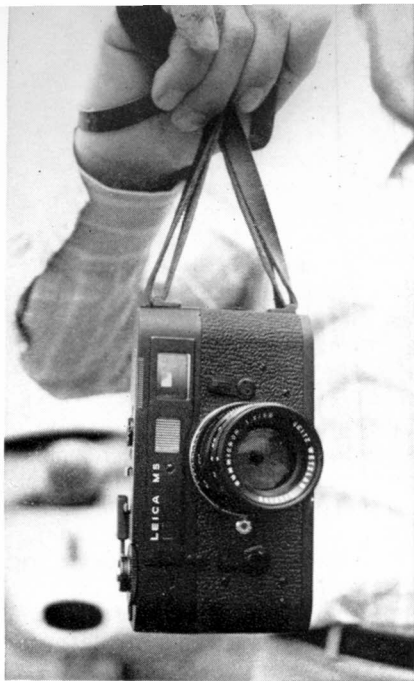
The holders for the strap of the Leica M5 are on one side.
