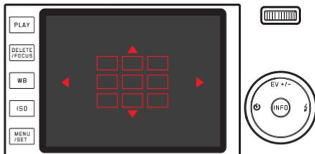
If required, you can concentrate the metering on any part of the image by selecting groups from either the three upper or lower or the four left or right AF fields:
