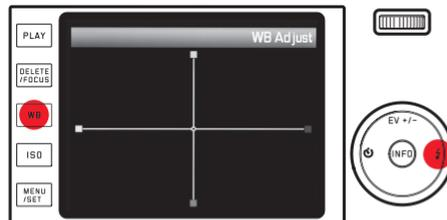
3. Use the direction pad to move the cursor - which is initially in the center - to the position that results in the required color reproduction in the monitor screen, i.e. towards the corresponding colored squares at the edges
