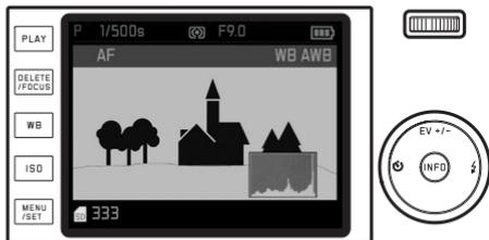
This form of representation – together with the impression of the picture itself – provides an additional quick and easy assessment of the exposure setting.
