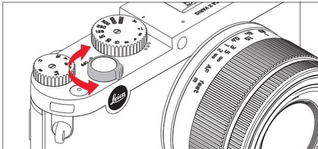
The Leica X is turned on and off using the main switch.
